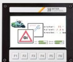
Warning and malfunction display faded in as a "Window"
