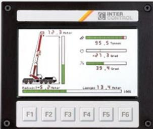
Interactive "set-up" of crane configuration
