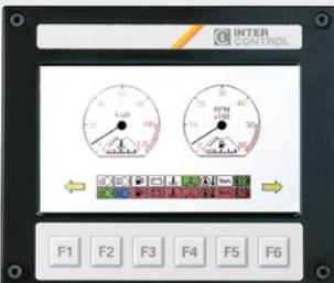
Pointer instrument – Display with engine data
